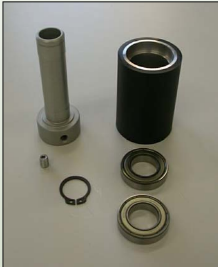
New counter pressure roller
