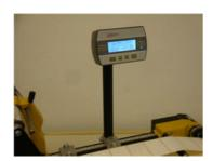
The port X103 is used to connect an external operator panel (in place of the original "potentiometer operator panel") to the labeler.
