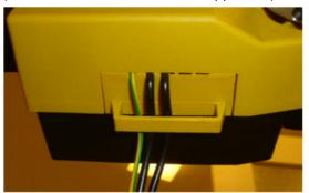
Special case **C4300-BUDGET**: the label scanner for this type of labeler will be connected directly to the main terminals on the main board (bottom). The label scanner cables are guided through the modular rail to the main board (entry of modular rail).
