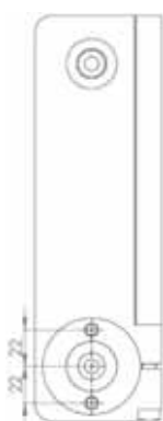
Adjusting bar. Fix with 2 x M6 and 1x M10. 2 x M6 and through holes for M10 provided by customer
