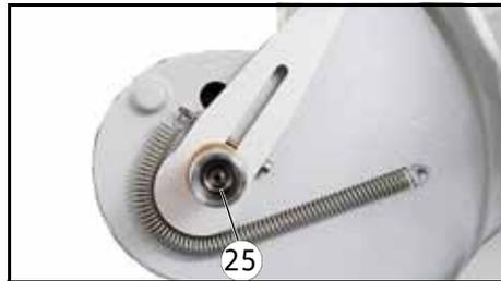
Fully tighten screw **25**, slowly loosen it thereafter until lever **20** is deflected approx. 45° (see following figure). So not change screw **25** thereafter.
