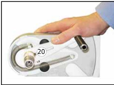
> Deflect lever **20** widely. Tighten clamping screw **18** slightly (not completely) such that the lever remains deflected after letting go but still can be turned manually. Make sure at the same time that clamping piece **17** is fixed on the shaft without play.
