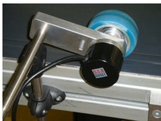
63.66mm wheel-Ø incremental encoder
